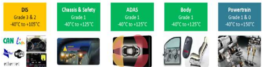
Figure 9: Examples of different grades of automotive semiconductor products based on application. SOURCE: TechSearch International
